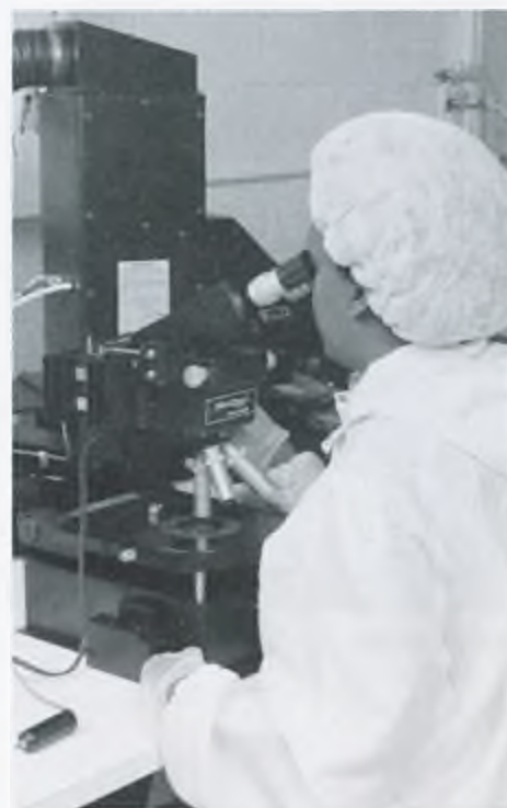
Research associate Konji Fekade operating deep ultra-violet mask aligner used for lithography.
