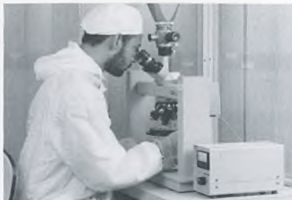
Graduate student Andre Cropper using microscope to examine lithography pattern on a crystal.
