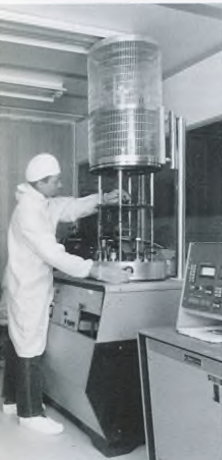
Research associate James Griffin working with electron beam evaporator.
