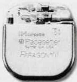
Paragon III, Pacesetter's newest dual-chamber pacemaker, weighs less than an ounce and is approximately 1/4" thick. The internal circuitry is controlled by an 8-bit microprocessor and operates at 2.8V. It is powered by a lithium-iodide battery.
