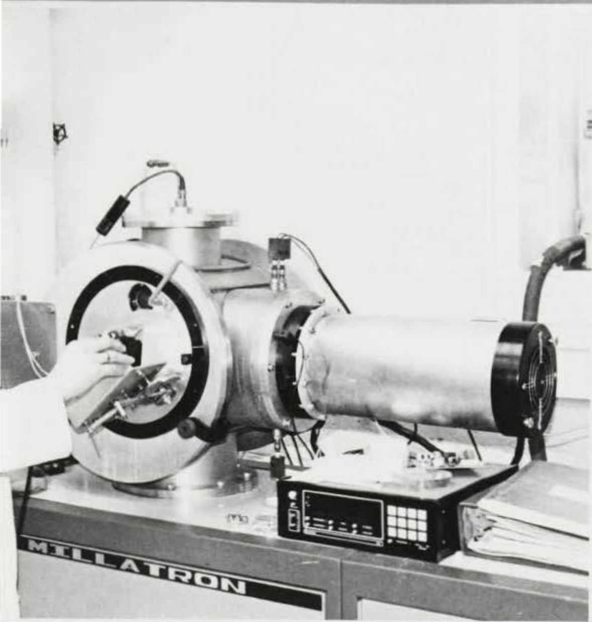
Angela Jones operates an ion milling machine which targets ions into a crystal's structure, to etch away a layer of the crystal.
