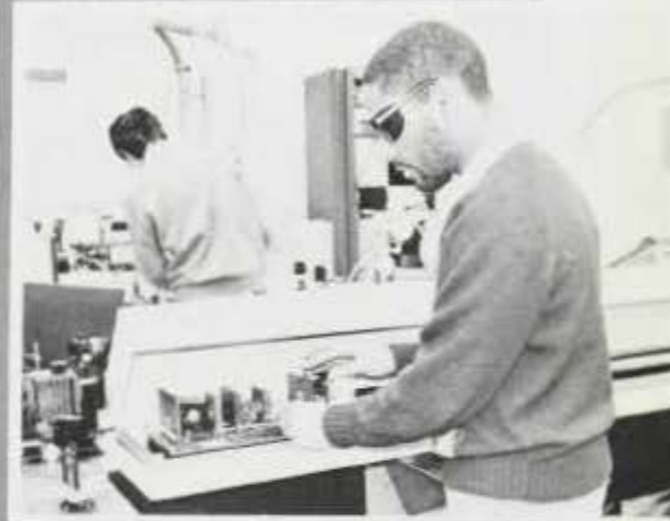
Eric Jones operates a laser system which is used for optical characterization of a semiconductor.
