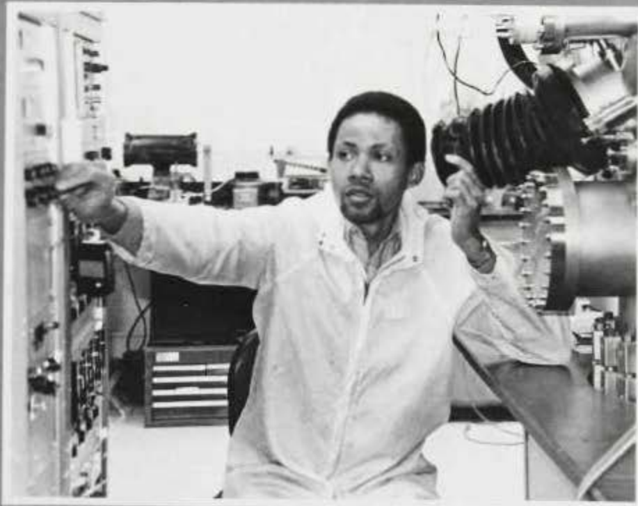
James Griffin, research associate, operates the Molecular Beam Epitaxy which is used to grow the crystals used for semiconducting devices.
