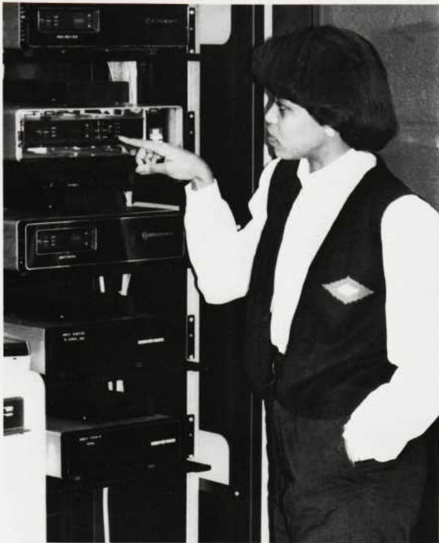
Connections. Cherrie Mallory points out that these modems help to link remote stations to the database.
