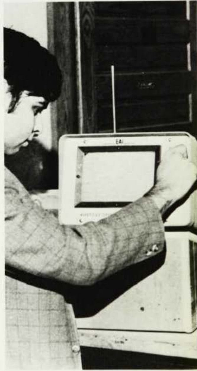
right: Analog computer simulates bend in an iron beam.
