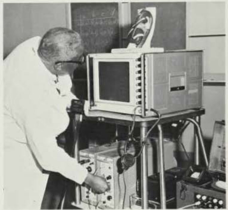
Dr. J. B. Johnson, in the Cardiovascular Research Laboratory, tests the "Electronic Patient" unit which is used to study the patient's heartbeat.
