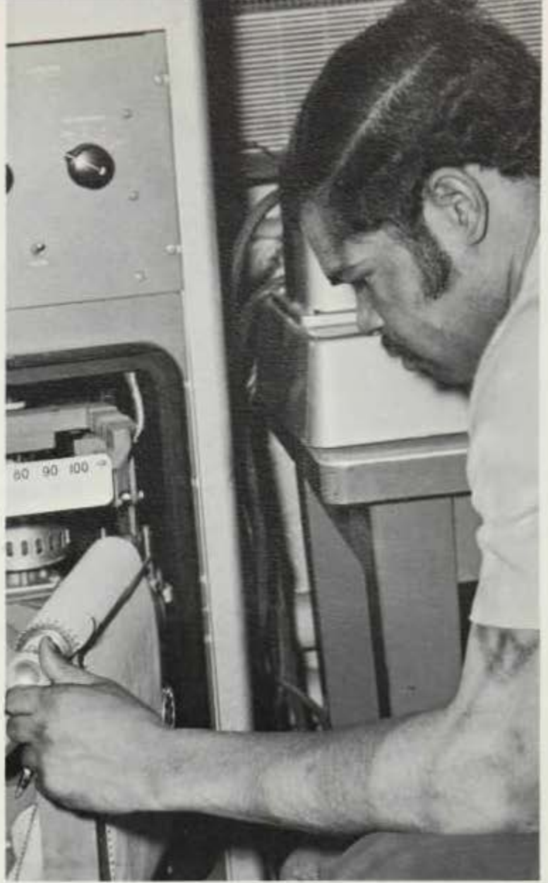
W. Johnson changes the tape on a spectrograph
