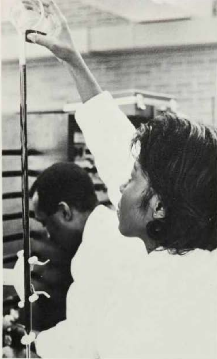
A third year student uses the buret to titrate her solution to the end point.
