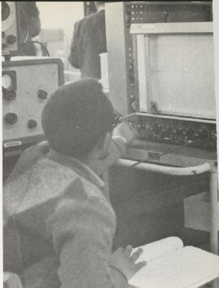
A new addition to the Electrical Department is this 10,000 cycle/sec. X, Y plotter.
