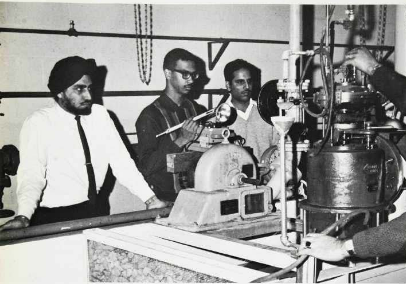
The causes and effects of the hydraulic jump in an open channel are being demonstrated to mechanical engineering students in their Fluid Mechanics Laboratory.
