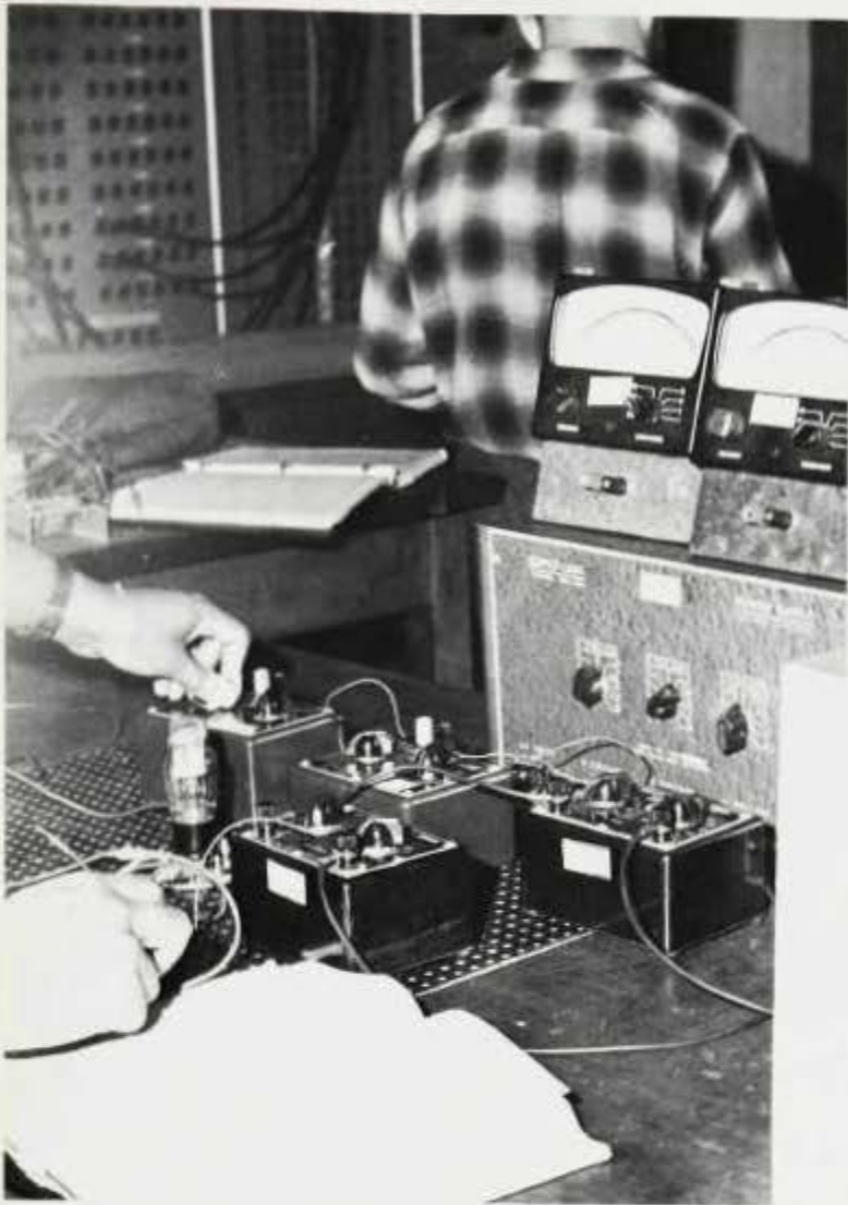
Senior Electrical Engineering student taking current and voltage readings with a varying resistance in a thyatron tube experiment, during an Electronics II lab.
