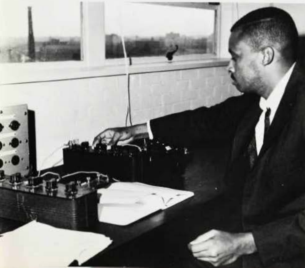
J. Johnson is varying the resistance by changing the potentiometer dials in order to determine the sensitivity of a galvanometer in the Electrical Measurements Lab.
