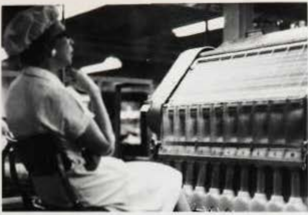
To fill twenty bottles of capsules per second is this machine's task.
